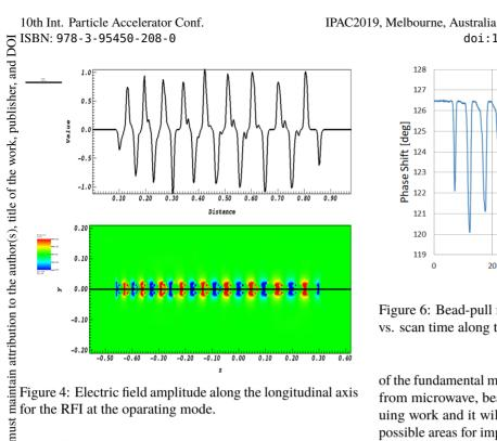
Figure 4: Electric field amplitude along the longitudinal axis
