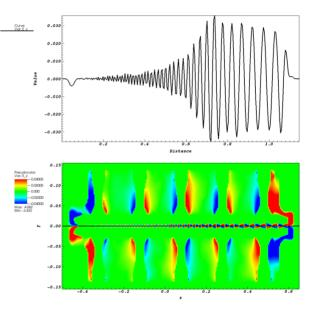
Figure 3: Amplitude of the longitudinal electric field corre sponding to the operating mode at 200 MHZ of the RFQ.
