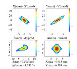
Figure 7: Phase spaces at the exit of the IH-EMQ (Au<sup>30+</sup>).
