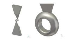
Figure 2: Model of the single cell and drift tube of IH-EMQ.
