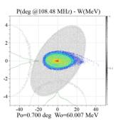
Figure 8: Longitudinal ellipse acceptance (shadow) of 60 MeV Au<sup>30+</sup> and emittance output from the RFQ (color).
