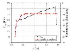
Figure 6: Gap voltage and synchrotron phase of IH-EMQ.
