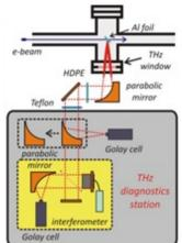
Figure 3: Setup of the CTR measurement.
