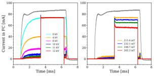
Figure 6: Chopped beam pulses for different chopper voltages (left) and different solenoid 2 strengths (right). The gray trace is the IS pulse as a reference.
