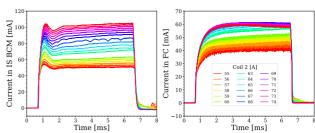
Figure 2: Beam pulse changes during a Coil 2 scan. Magnetron power, Coil 1 current, Coil 3 current, and  $H_2$  injection were kept to 500 W, 120 A, 217 A, and 3.5 sccm.
