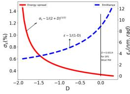
Figure 5: Parameterization of the emittance (blue) and energy spread (red) with D for the effect of RW in addition to DW at 20 GeV.
