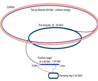
Figure 1: Layout of the FCC- $e^+e^-$  injector complex [1].
