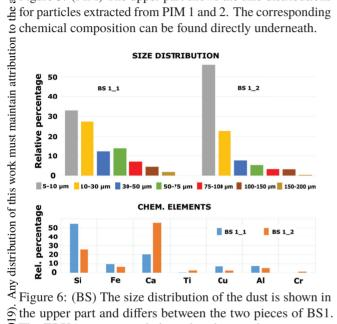
$\widehat{\mathfrak{D}}$  the upper part and differs between the two pieces of BS1. S The EDX spectra revealed similar elemental composition <sup>(2)</sup> for the dust found in BS1 1 and BS1 2, but the peaks in Si and Ca seem complementary.
