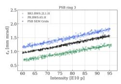
Figure 1: Horizontal emittance versus intensity, as measured with the PSB WS (green), the PS WS (blue) and the SEM grids in the BTM line (black).
