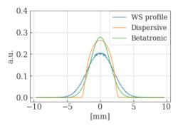
6 Figure 5: Measured beam profile from the PSB WS in com-Sparison to the dispersive and betatronic profiles computed with the full deconvolution algorithm.
