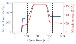
Figure 2: The 160 MeV flat-top energy cycle. The dashed lines indicate injection and extraction times (at 275 ms and 805 ms, respectively).
