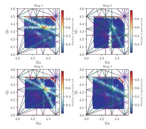
Figure 3: Static tune scans for each ring of the PSB with multipoles off, where the tune values are the measured ones.
