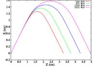
Figure 7: Trajectories of proton beam with four energies inside one bending magnet of the entrance phase shifter with large fringe field region.
