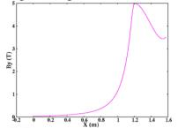
Figure 8: Middle plane magnetic field profile inside the bending magnet of the entrance phase shifter.
