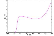
Figure 6: Middle plane magnetic field profile inside the bending magnet of the exit phase shifter.
