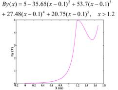
Figure 10: Middle plane magnetic field profile inside the bending magnet of the exit phase shifter.
