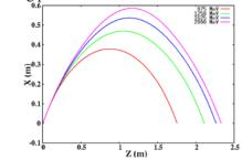
Figure 5: Trajectories of proton beam with four energies inside one bending magnet of the exit phase shifter.
