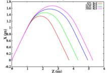
Figure 9: Trajectories of proton beam with four energies inside one bending magnet of the exit phase shifter with large fringe field region.
