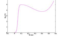
Figure 4: Middle plane magnetic field profile inside the bending magnet of the entrance phase shifter.
