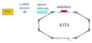
Figure 5: A schematic configuration of the basic set-up with the LAPPD diagnostics; a single electron passing through the undulator will generate photons which can be spectrally filtered to reduce noise, then magnified with an optical telescope, and detected with the LAPPD detector.
