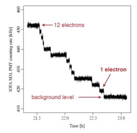
Figure 2: A measured photo-multiplier signal from a synchrotron radiation monitor after the bend magnet. One can clearly see finite jumps in the average proton count rate level as the number of trapped electrons becomes small, until a single electron is left in the IOTA storage ring.
