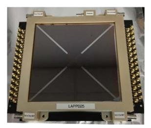
Figure 4: A photograph of the LAPPD detector, which features a 200×200 mm active area and 100 ps temporal resolution.
