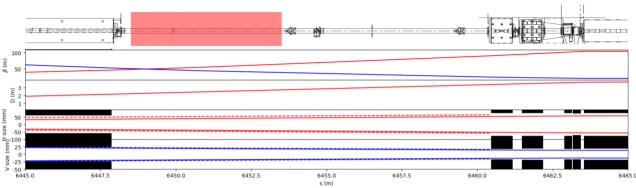
Figure 2: Layout of the SPS section 621 on top with the foreseen position of the laser cavity in red. Bellow, optical functions and beam sizes are shown in red for the horizontal plane and in blue for the vertical one. Dotted lines presents the minimum physical aperture required for compatibility with the other beams accelerated in the SPS.
