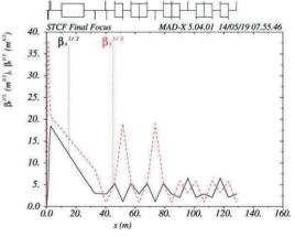
Figure 4:  $\beta$  function of 1/2 final focus section.
