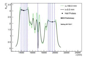
Figure 2: Magnitude of the of the magnetic field along the length of the cooling channel. Hall probe measurements are included as verification, and the field strength at the position of the hall probes is shown in green (160mm off axis). The central cusp is due to the magnetic field flip.
