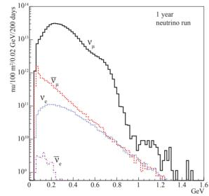
Figure 3: Neutrino energy distribution at an arbitrary distance of 100 km on–axis from the target station, for 2.5 GeV protons and positive horn current polarity.
