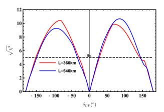
Figure 4: CP violation discovery significance versus  $\delta_{CP}$  for two baselines, 360 km and 540 km corresponding to the two active mines Zinkgruvan and Garpenberg, respectively.
