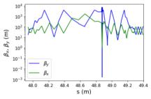
Figure 1: Beta functions near the IP of the 182.5 GeV lattice.
