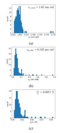
Figure 3: Distribution of (a) horizontal emittance, (b) vertiunder the terms of the CC cal emittance, and (c) coupling ratio of the corrected ttbar lattices. The errors introduced are summarized in Table 2.
