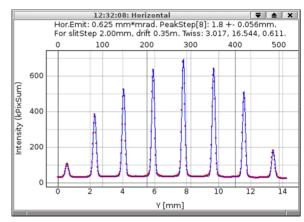
Figure 3: Emittance measurement of 0.75 nC bunch with slits.
