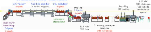
Figure 1: Layout of the CeC proof-of-principle system at IP2 of RHIC.
