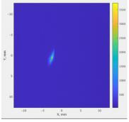
Figure 2: Image of the compressed and accelerated beam in the dogleg profile monitor. The dispersion is 1.2 meters and beam energy spread is  $3x10^{-3}$ .
