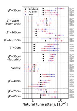
Figure 2: Measured and predicted tune jitter for various optics at 6.5 TeV, from [19]. Optics with  $\beta^*$  < 10m are ATS.
