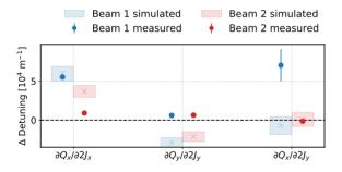
Figure 6: Measured and predicted change in the natural amplitude detuning coefficients from switching on crossing angle in IR5 at  $\beta^*$ =30 cm.
