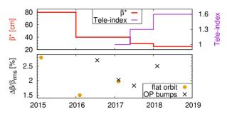
Figure 1: Run 2 at a glance:  $\beta^*$ , tele-index (top) and rms  $\beta$ -beating (bottom) averaged over the two planes and two beams, with and without operational (OP) crossing angle. Note that the 2016 measurement with OP bumps misses one plane out of four.
