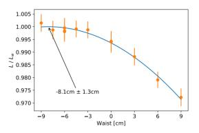
Figure 3: Luminosity versus waist scan as proof-of-principle for accurate waist position measurement, from [21].
