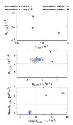
Figure 5: Comparison between beam-based and magnetic measurement-based IR non-linear corrections in 2018.
