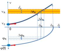
Figure 2: Particle's synchrotron oscillations with maximum amplitude  $\delta_0$  crossing resonance at  $\nu R=p/2$  with the stopband width of  $J_n$ .
