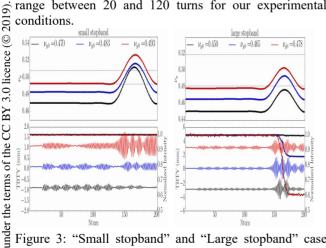
Figure 3: "Small stopband" and "Large stopband" case Turn-by-turn beam parameters (upper plot: calculated y-tunes with dashed lines indicating borders of the stopband, lower plot: BPM measured TBT y-position on left axis and normalized beam intensity on right axis) for the three separate experiments with different initial tunes.
