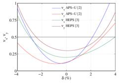
Figure 1: Fractional tune shift with momentum deviation as presented in [2, 3].
