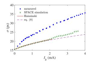
Figure 2: Intensity-dependent bunch length.
