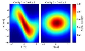
Figure 2: Headtail monitor acquisitions comparing two cases which show the CCs in phase (left) and cancelling (right).
