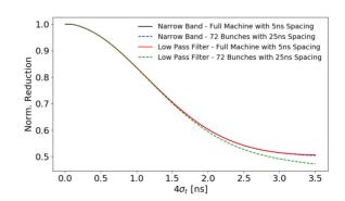
Figure 1: The normalised BPM readout as a function of bunch length for different types of filters and beam parameters. The bunch length at 26 GeV is  $4\sigma_t \approx 2.9$  ns and at 270 GeV it is  $4\sigma_t \approx 1.4$  ns.
