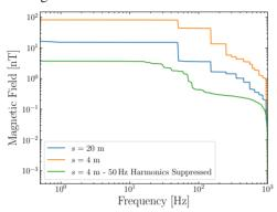
Figure 6: Smallest and largest integrated magnetic field measured in CLEAR. *s* is the position along the beamline from the electron gun.
