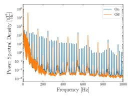
Figure 7: Magnetic field power spectrum measured at the XBOX-3 test stand on 06/12/18 with and without the klystron running. The klystron was operating at 16.7 Hz.
