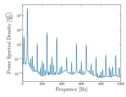
Figure 2: Average power spectral density measured over one minute underneath the power lines at 15:02 on 10/09/18.
