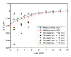
Figure 2: Measured mean energy change per structure as a function of the gap compared with the simulated results. The bunch has a charge of 200 pC, a Gaussian longitudinal shape with  $\sigma$  equal to 1.1 mm (measured electron bunch length).
