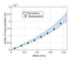
Figure 3: Orbit deviation of the electron bunch as a function of the transverse offset in the structure (kick factor) compared to the simulations (assumed charge in a range between 160 pC and 200 pC).
