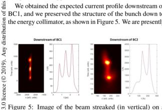
Figure 5: Image of the beam streaked (in vertical) on a BZ screen downstream of BC1 at 300 MeV (left), and at the energy collimator at 5.8 GeV (right plot), and corresponding current profiles. In this case we present the measurements the terms of the done using the flat-top distribution.
