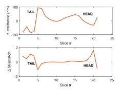
Figure 6: Variation of the emittance and mismatch along the bunch in the configuration with the passive structures closed (gap = 3 mm) with respect to the case where the structures are open.
