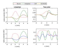
Figure 1: Wake potential obtained assuming Gaussian and flat-top bunch profiles. We assumed a Gaussian bunch with  $\sigma = 0.9$  mm and a flat-top distribution with FWHM of 10 ps. For both cases we used a bunch charge of 200 pC, which is the maximum design charge of SwissFEL.
