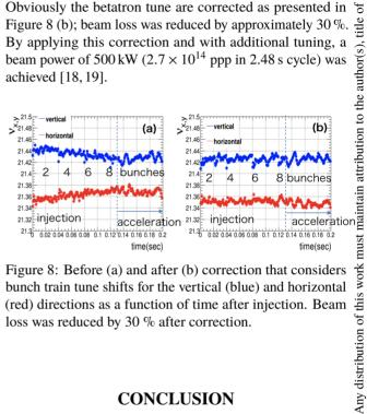
Figure 8: Before (a) and after (b) correction that considers bunch train tune shifts for the vertical (blue) and horizontal (red) directions as a function of time after injection. Beam loss was reduced by 30 % after correction.
