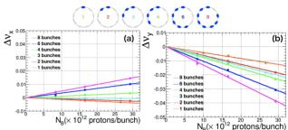
Figure 1: Measured tune shifts as a function of the bunch intensity, horizontal (a) and vertical (b) directions. The linear fits are also shown.
