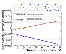
Figure 2: Measured tune shift slopes as a function of the number of bunches with fitted lines. The sign of the tune shift slope for horizontal and vertical directions is opposite.
