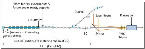
Figure 1: Schematic of ARES Linac with Bunch Compressor and matching section into LWFA \*sumera.yamin@desy.de
