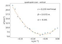
Figure 9: Results of the quad scan in vertical plane with  $^{12}C^{6+}$  beam at 1450 MeV/u.
