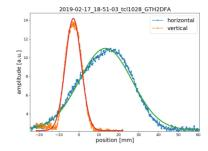
Figure 8: Beam profiles obtained with CUPID.
