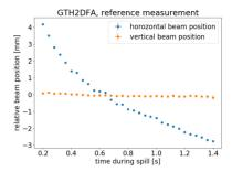
Figure 4: Movement of the beam during the spill.
