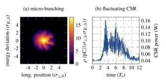
Figure 1: (a) The CSR self-interaction of the bunch causes the formation of micro-structures in the longitudinal phase space density. (b) Their continuous variation leads to fluctuations in the emitted CSR power. The illustrated dynamics are simulated with the VFP solver Inovesa.
