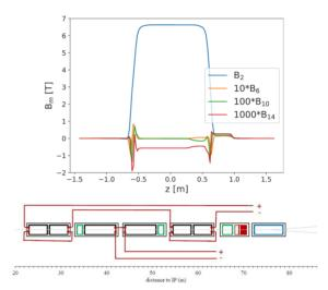
Figure 1: Normal harmonics sampled at  $\Delta z = 2$ mm for the prototype of the IT quadrupole (top). IT powering scheme (bottom). Courtesy of E. Todesco and S. Izquierdo Bermudez
