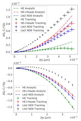
Figure 2: Amplitude detuning for the x-plane (top) and the y-plane (bottom). The b<sub>6</sub> corrector (called MCTX) has been switch OFF.
