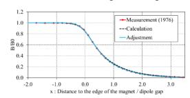
Figure 6: Fringed field of the dipole: the 1976 measurement (in red), the OPERA calculation (in black), and the fitting of the experimental data (in blue).
