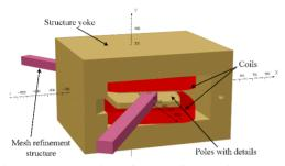
Figure 3: Conception of the H-dipole with OPERA.
