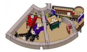
Figure 1: Scheme of the ISOL facility ALTO: 1. 50MeV Electron LINAC, 2. Target ion source vault, 3. Mass separator, 4. Transfer lines, 5. and 6. experimental setups in operation and under construction.
