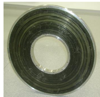
Samples of magnetic alloy tape wound cores, measured for the SIS bunch compressor project. The ring to the left is a FineMet core, produced by Hitachi in Japan. The right one is a VitroVac core,
