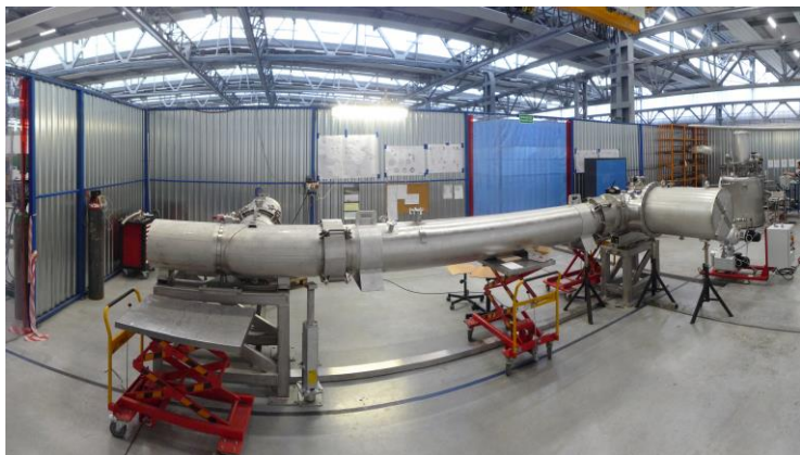
First cryogenic bypass line with integrated bus bar system shipped and tested
