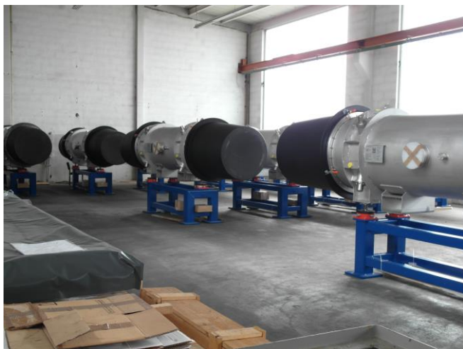
Fast ramped (4 T/s) s.c. dipole magnets Series production started. 21 modules delivered.
