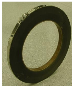
Samples of magnetic alloy tape wound cores, measured for the SIS bunch compressor project. The ring to the left is a FineMet core, produced by Hitachi in Japan. The right one is a VitroVac core,
