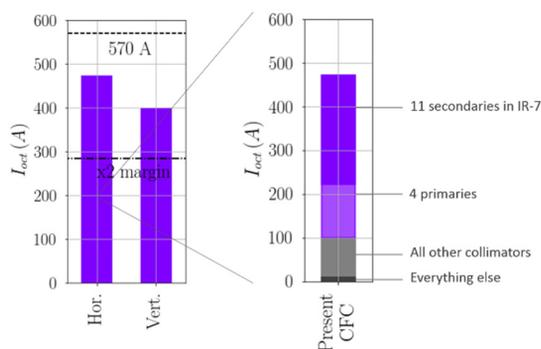
Figure 2: Impedance of LHC collimators has to be reduced for the Hi-Lumi upgrade. It is responsible for nearly all the octupole current required to stabilize the beam at the top energy, with ~50% coming from 11 secondary collimators.  $E = 7$  TeV, BCMS beam, Ultimate operational scenario [9].
