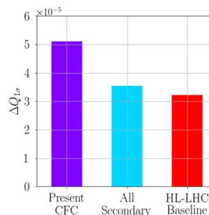
Figure 5: Threshold rms detuning required to stabilize the most unstable mode reduces significantly with low-impedance collimators. Most critical, horizontal plane.
