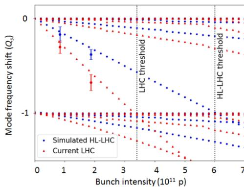
Figure 7: Collimator upgrade is expected to increase the TMCI threshold at the top energy by nearly a factor of two in HL-LHC (blue) compared to LHC (red). The measured mode frequency shifts (error bars) are in good agreement with simulation predictions (dotted lines) [17].
