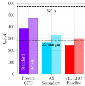
Figure 6: Novel coatings provide sufficient stability margin both for standard and BCMS beams. For a standard beam  $\sim 120$  A is gained by upgrading all the secondaries in IR7 to Mo-coated MoGr and additional  $\sim 30$  A – by replacing the two baseline primary collimators with MoGr. The situation in the most critical, horizontal plane is shown.
