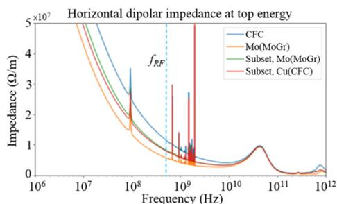
Figure 4: Low-impedance secondary collimators decrease the machine impedance by 30% at the frequencies  $\sim 1$  GHz, relevant for the single-bunch coherent dynamics. Coating a subset of four collimators provides a half of the reduction. Chromaticity  $Q' = 0$ ; 7 TeV; narrow spikes near 1 GHz correspond to the higher order modes (HOMs) of HL-LHC crab cavities. RF frequency shown by a dashed line.
