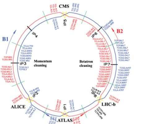
Figure 1: Schematics of the LHC collimation layout [2].
