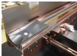
Figure 3: The jaw of the prototype collimator that was used to study different coatings in LHC [12].
