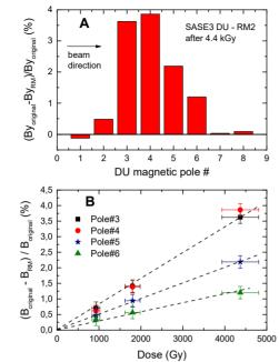
Figure 3: Magnetic degradation on the (A) SASE3 DU and (B) for poles #3 to #6 as function of absorbed doses.
