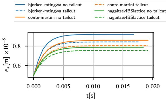
Figure 2: Horizontal emittance evolution using a Coulomb logarithm with and without a tail-cut procedure, for different IBS models (Bjorken-Mtingwa [2] (blue), Conte-Martini [6] (orange) and Nagaitsev approximation [7] (green)).
