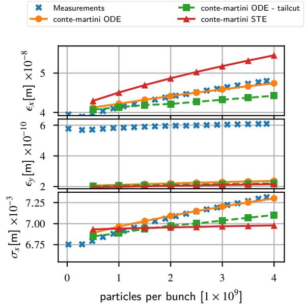
Figure 4: Comparison MLS measurements (blue) with ODE simulations (with (red) and without (orange) tail cut) and particle tracking simulations (green) using Conte-Martini as IBS model.
