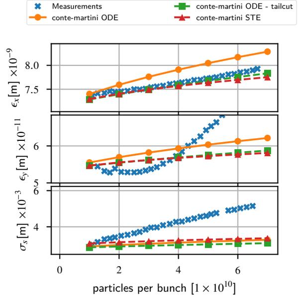
Figure 3: Comparison BESSY II measurements (blue) with ODE simulations (with (red) and without (orange) tail cut) and particle tracking simulations (green) using Conte-Martini as IBS model.
