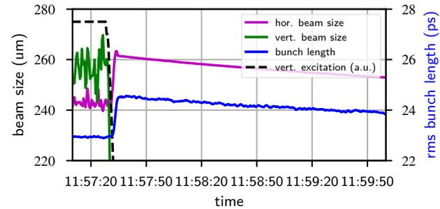
Figure 1: MLS: vertical noise excitation (black dashed), bunch length (blue), horizontal (magenta) and vertical emittance (green) measurement with and without vertical noise excitation
