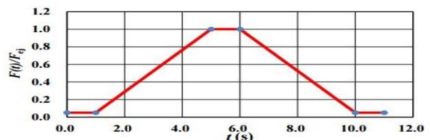
Figure 1: The magnetic field cycle of the Booster.
