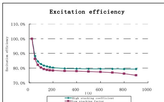
Figure 5: The excitation efficiency calculated by excitation curve.
