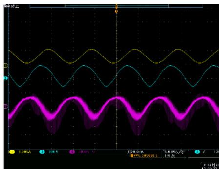
Figure 5: The output current (ch1), the output voltage (ch2) and the voltage fluctuations of the DC-Link for QPS3.
