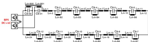
Figure 1: Resonant network of the RCS Dipole PS.
