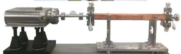
Figure 4: 750mm long strip-line kicker prototype.
