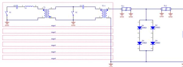
Figure 9: DSRD pulser schematic.
