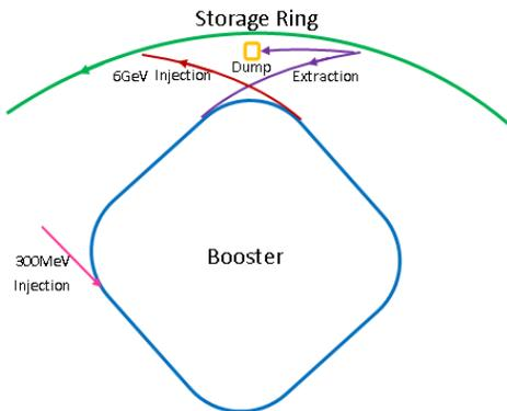
Figure 1: HEPS injection and extraction system layout.
