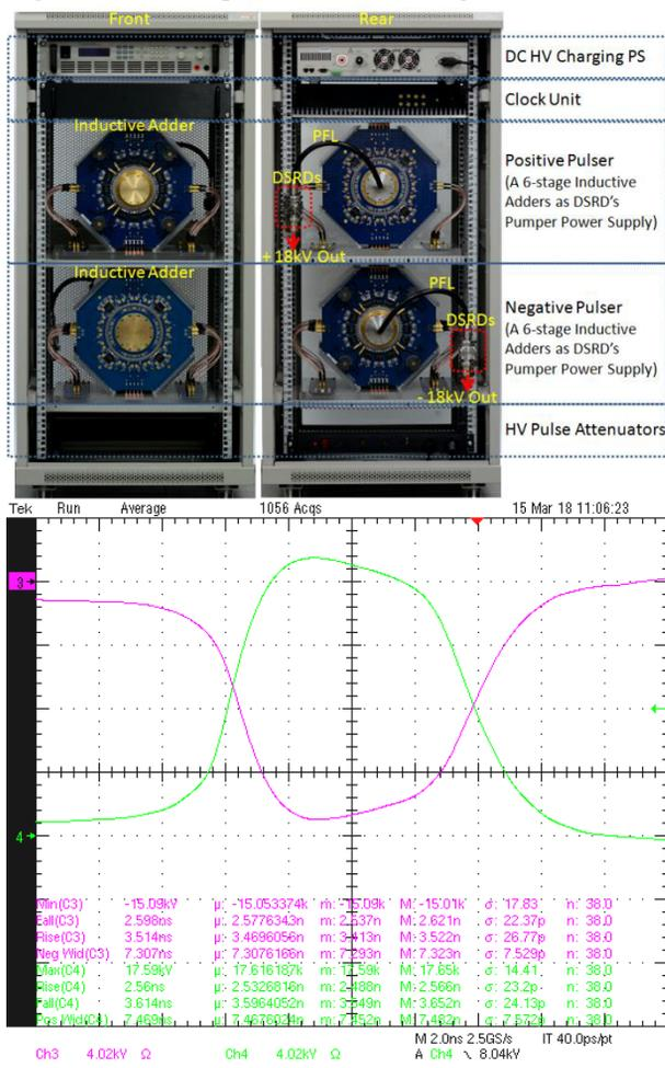
Figure 11: DSRD pulser prototype and testing result.
