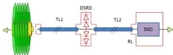
Figure 10: DSRD pulser structure.
