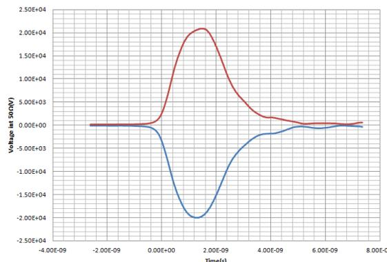
Figure 8: Kicker prototype HV test waveform.
