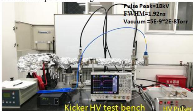
Figure 7: Kicker prototype HV test set up.
