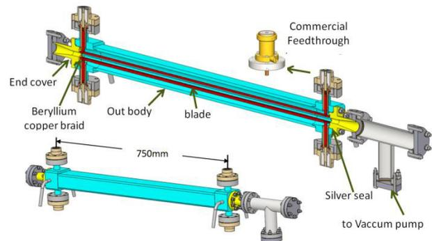
Figure 3: 3D mechanical assembling diagram of kicker.
