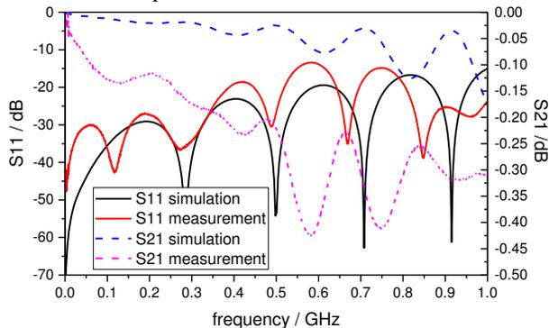
Figure 5: Testing and simulation S parameters.
