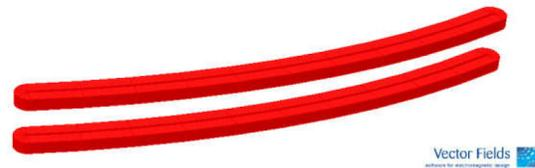
Figure 3: 3D model of one pair of trim coil.
