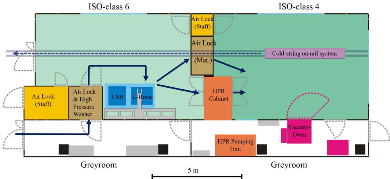
Figure 1: Sketch of the HIM-cleanroom. The ISO-class 6, -class 4 and greyroom areas are shown, as well as the different features such as air locks for personnel and objects, large ultrasonic (USB) and conductance rinsing (C-Rinse) baths with their crane, a high pressure rinsing (HPR) cabinet, vacuum oven and mounting rail for cold-string assembly and transportation. Typical transfer paths for objects and material (blue arrows) are depicted.
