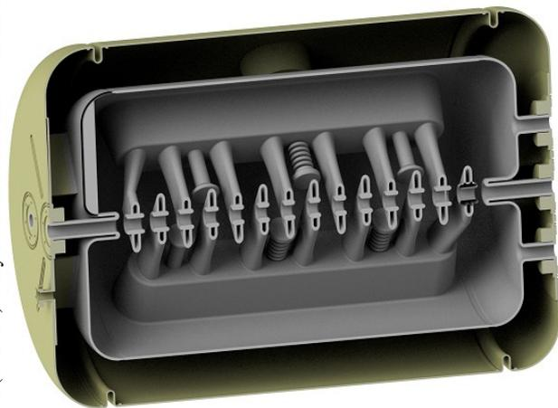
Figure 4: Sectional view of the first 217 MHz CH cavity for the cw linac at GSI; 10 cm off beam axis two openings from each side for additional rinsing of the four sector quadrants are available.
