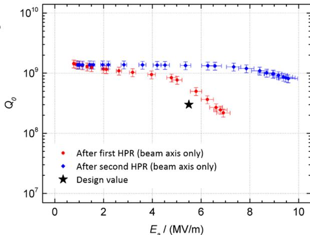
Figure 3: Measurements of  $Q_0$  and  $E_a$  at a CH-cavity at 4 K; between first (red) and second (blue) test another HPR procedure has been performed [4].
