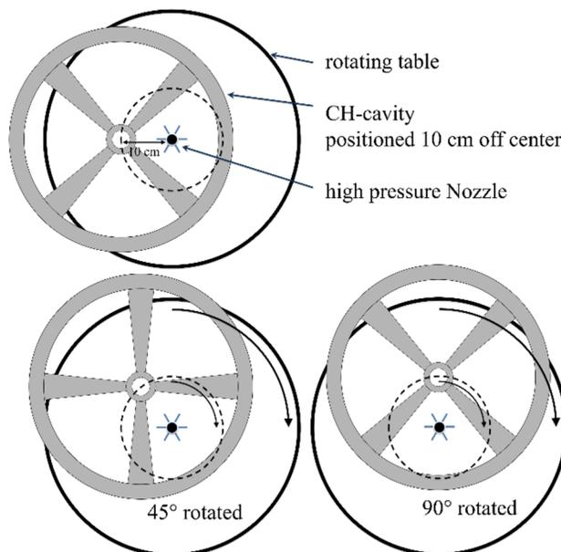
Figure 5: Schematic illustration of the high pressure rinsing process at one sector quadrant of a CH-cavity.
