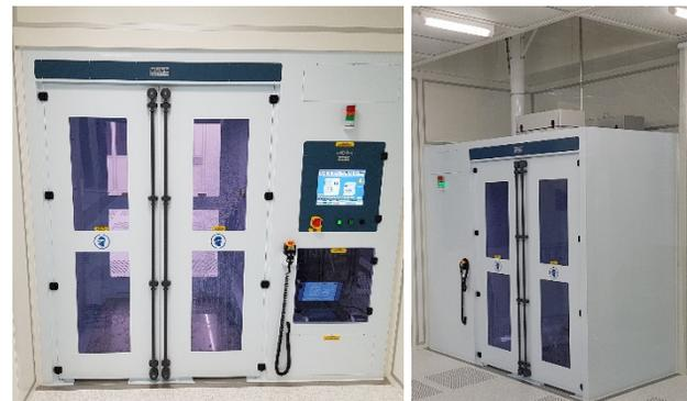
Figure 2: HPR cabinet: View from ISO-6 access side for loading (left) and from ISO-4 for unloading (right). The lever with the wand is visible.
