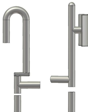
Figure 1: Hook-type coupler (left) and Probe-type coupler (right)
