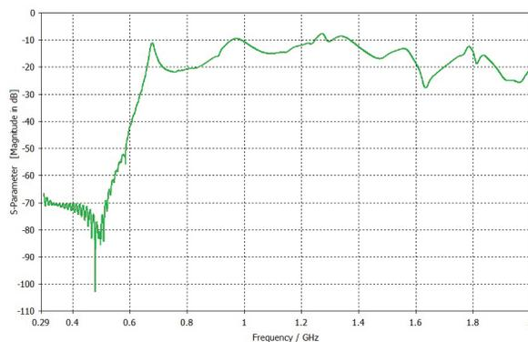
Figure 4: S21 parameter of the Hook-type coupler simulated with the simplified model.
