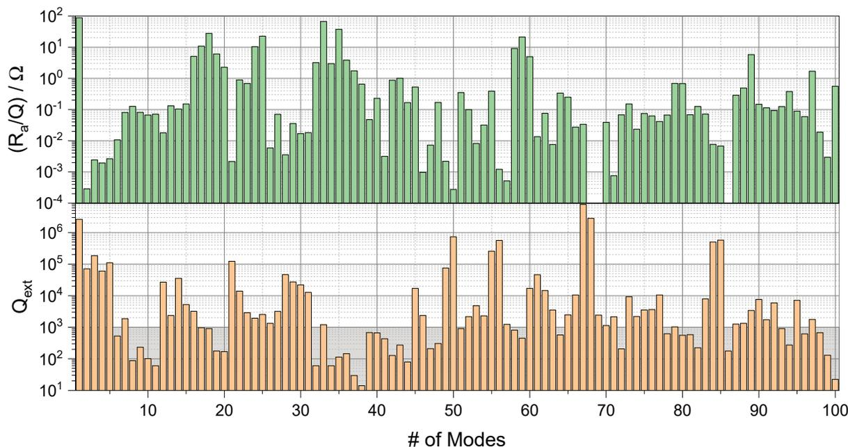
Figure 6: Shunt impedance of the first 100 modes (top) and the corresponding external quality factors (bottom) with the threshold of 1000 plotted in light grey in the background.
