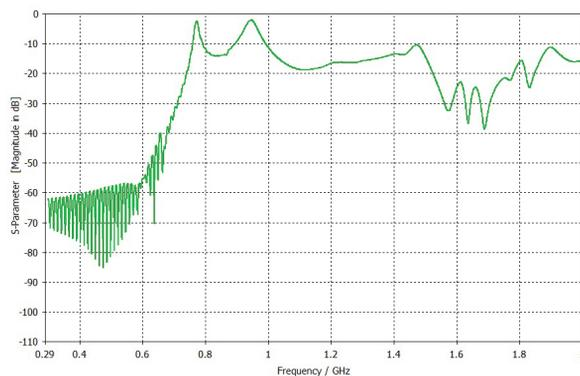
Figure 5: S21 parameter of the Probe-type coupler simulated with the simplified model.
