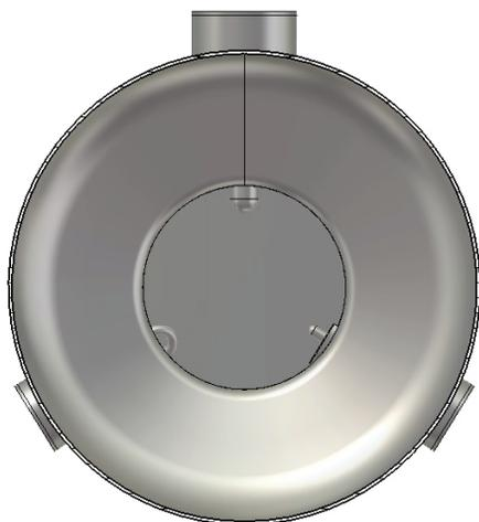
Figure 2: Cross section along the xy plane of the cavity. The FPC is located at the top and the HOM couplers are located at the bottom.
