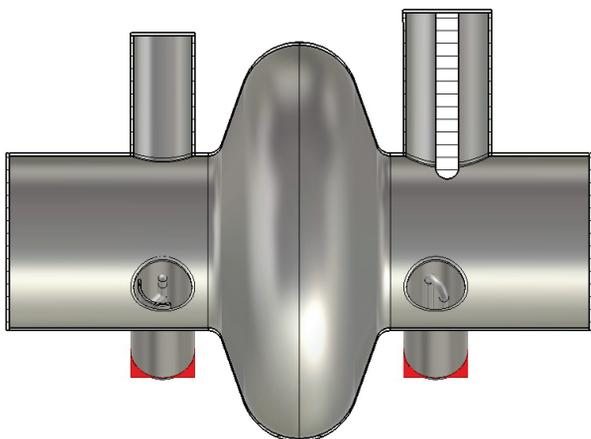
Figure 3: Cross section along the beam axis of the cavity. One of each type of HOM couplers is placed left and right from the cavity.
