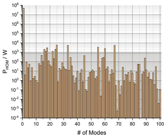
Figure 7: Deposited power in one HOM coupler of the first 100 modes with a threshold of 800 W plotted in light grey in the background.
