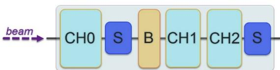
Figure 1: Proposed layout of the first CW-linac cryomodule comprising 3 CH-DTLs (CH0, CH1 and CH2), S – solenoid and B – re-buncher cavity.
