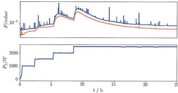
Figure 7: First phase of conditioning process with several degassing events at the input coupler.
