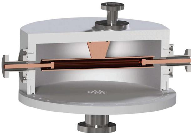
Figure 4: Rendering of the quarter-wave resonator alike structure.
