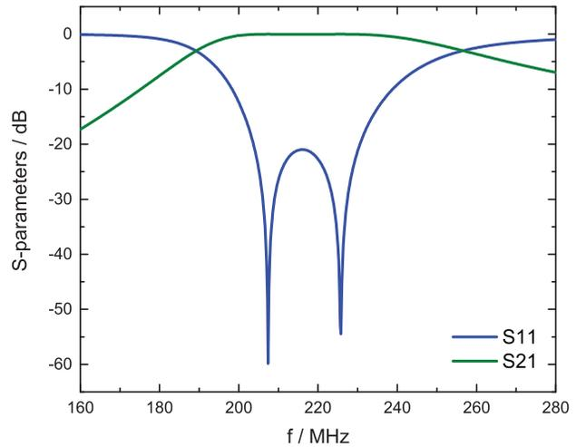
Figure 5: Transmission and reflection parameters for the test bench structure.
