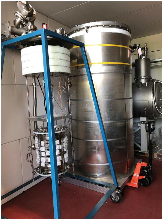
Figure 3: Vertical test environment for further measurements of the cavity.
