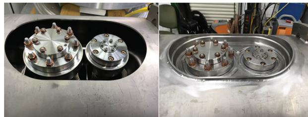
Figure 2: Left: Separated helium vessel comprising membrane bellows. Right: Replacement component.
