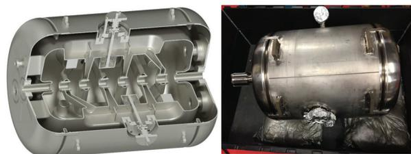
Figure 1: Left: Rendered cross section of the 325 MHz CH-Cavity. Right: Cavity with fixed helium vessel.
