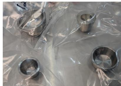
Figure 2: Four different tungsten crucible sizes.
