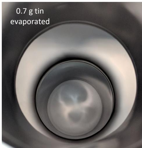
Figure 4: Cavity coating after coating parameter development with no apparent non-uniformities
