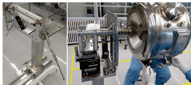
Figure 4: Beam pipe end-subassembly tooling.
