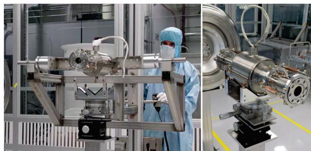
Figure 3: Tools for solenoid subassembly.
