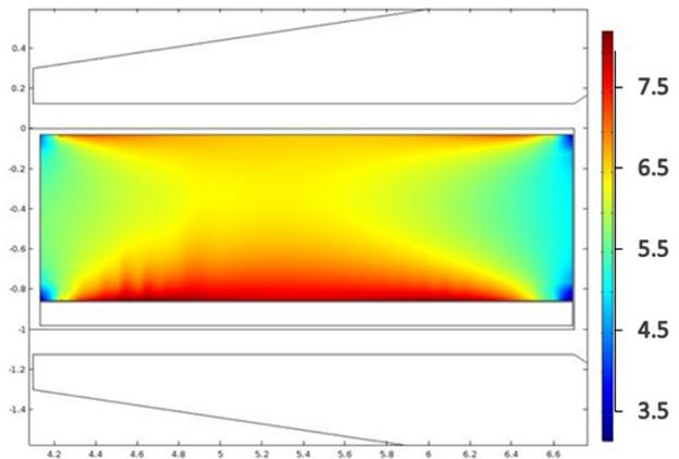
Figure 6: Modelling results for permeability in the garnet when the solenoid bias is  $\sim 1000$  A-turns and the cavity resonant frequency is  $\sim 70$  MHz.
