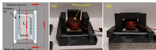
Figure 2: Sketch and photographs of the witness sample test setup.
