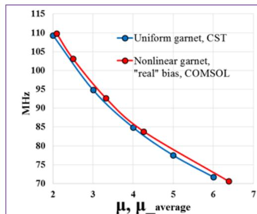
Figure 7: Modelling results for cavity frequency as a function of the garnet permeability. In one case (CST), it was assumed that the permeability in the garnet was uniform. In another case (COMSOL) it was not uniform.
