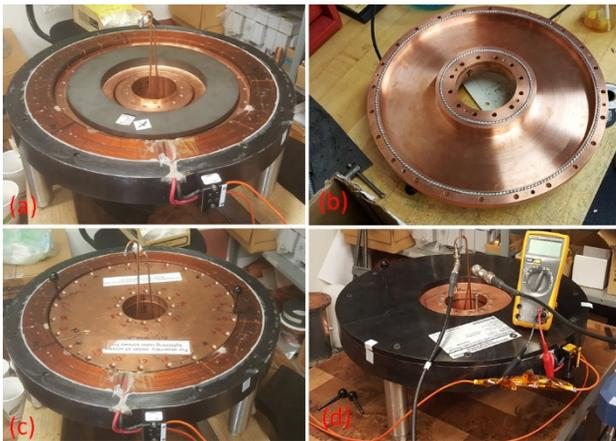
Figure 5: Photographs of the tuner ring test cavity (a) with tuner ring and shorting lid off, (b) inside of shorting lid, (c) with shorting lid on, (d) fully assembled with flux return top in place.
