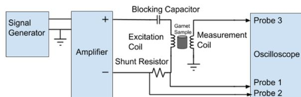
Figure 3: Circuit used in the witness sample permeability measurements.
