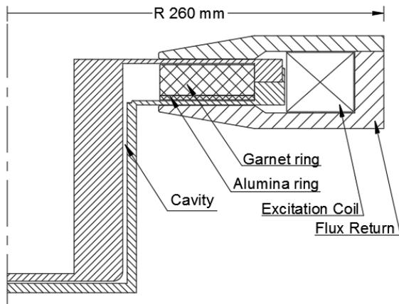
Figure 4: Schematic of the tuner ring test cavity with magnet.
