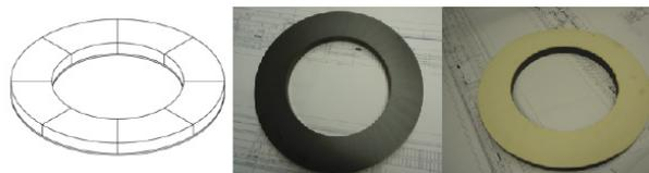
Figure 1: Drawing and photographs of the garnet and alumina sides of a tuner ring. The ring OD is 13.386".
