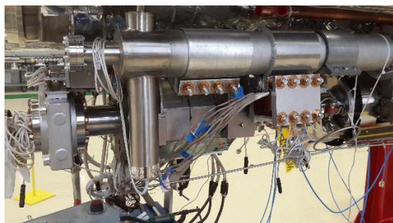
Figure 3: Magnet side view with heat sinks installed.
