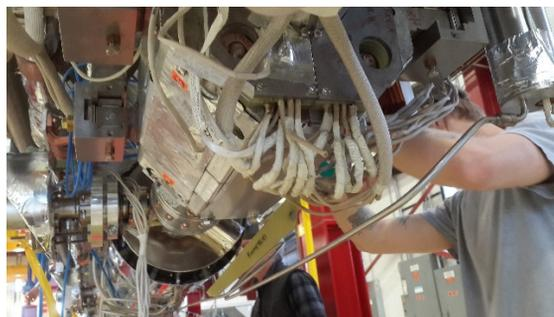
Figure 2: Magnet with leads and instrumentation wiring.
