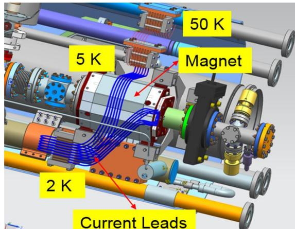
Figure 1: Superconducting magnet in the Cryomodule.
