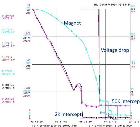
Figure 5: The magnet cooling down to the superconducting state.
