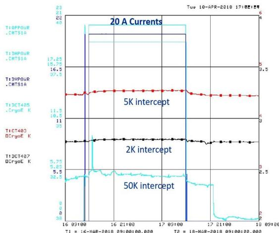
Figure 6: Full power 24 hours test.
