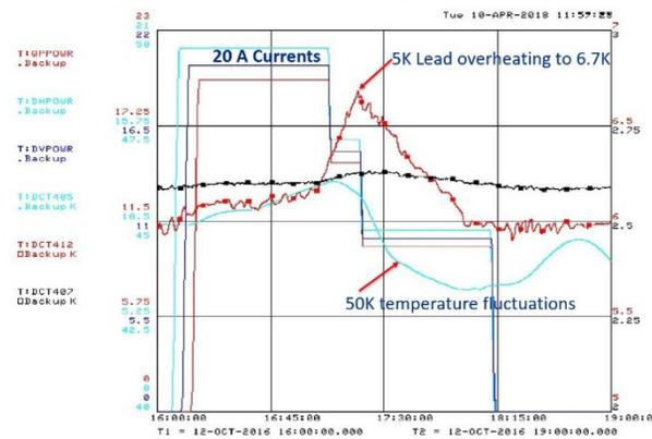
Figure 4: Current leads temperature rise at 20 A in all coils.
