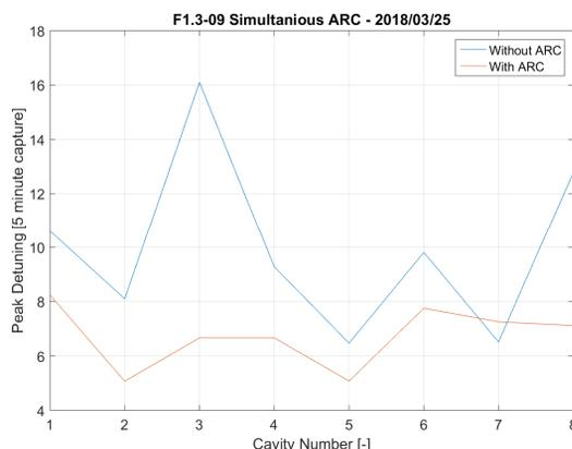
Figure 5: Peak detuning during 5 minute captures (at 1 kHz) by cavity with and without ARC.
