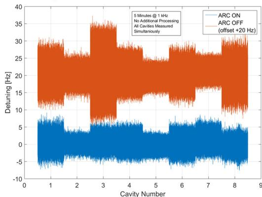
Figure 4: Short captures of all eight cavities with (blue) and without (orange + offset) ARC.
