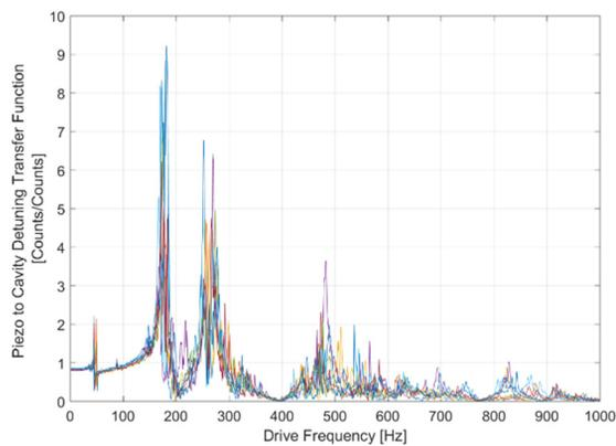
Figure 1: Eight cavity transfer functions measured simultaneously at CMTS-1 on F1.3-09.
