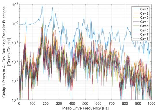
Figure 2: Cavity 1 piezo to all cavities detuning transfer function measured on F1.3-09.
