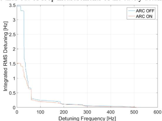
Figure 3: Integrated RMS detuning with and without ARC on only cavity 8 of F1.3-09.
