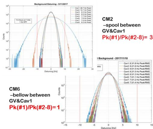
Figure 8: Microphonics measurements of cryomodule F1.3-02 and cryomodule F1.3-06. F1.3-02 had no gate valve/cavity 1 modifications. F1.3-06 had the extended tuner arms and bellow between gate valve and cavity 1.
