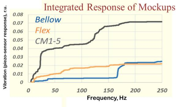
Figure 3: Summary of the warm study with cavity#1 mock-up. Integrated response when 300mm He return pipe strike with hammer.
