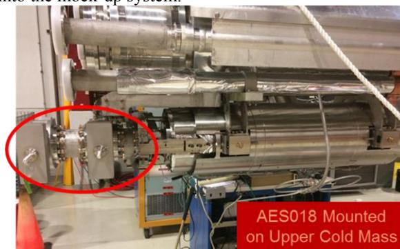
Figure 2: Picture of the mock-up for warm study of the proposed gate valve/cavity#1 modifications.
