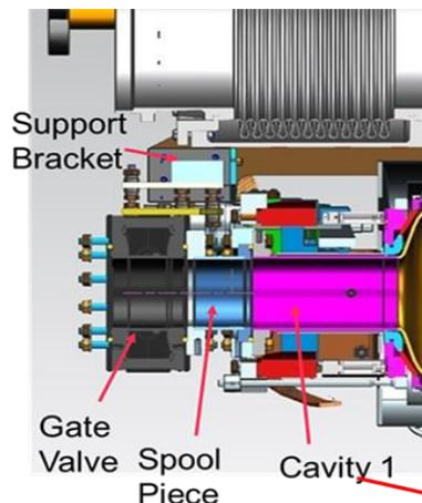
Figure 1: Picture of the “standard” interface between cavity#1 and gate valve.
