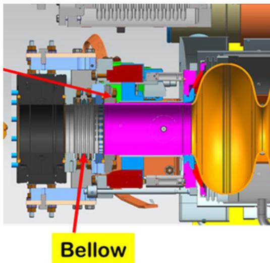
Figure 4: Drawings of the modification of the gate valve/cavity 1 interface, including short bellows introduced between cavity beamline flange and gate valve.
