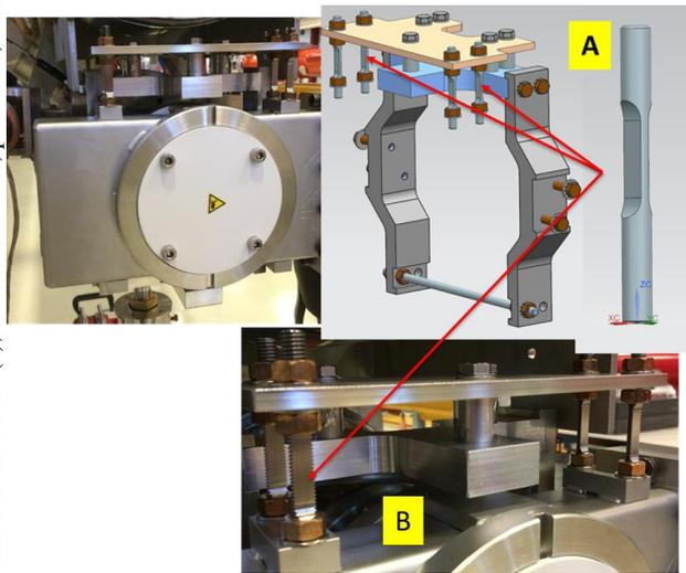
Figure 7: Tuner modification with flexible joints. (A) 3-D model of the cage to support gate valve. (B) Photo of the gate valve mounted with flexible rods.
