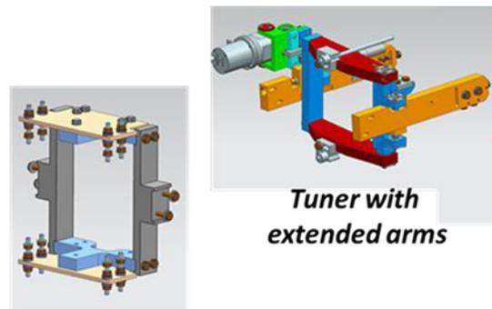
Figure 5: 3-D model of the LCLS II tuner with extended arms (right) and gate valve support bracket (left).
