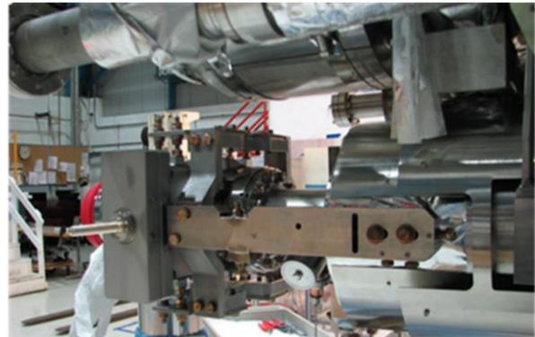
Figure 6: Picture of the cavity 1 and gate valve assembled on cryomodule 6 with bellows. Extended tuner arms attached to the He vessel of the cavity 1. The support cage is mounted on the arms and supports the gate valve.
