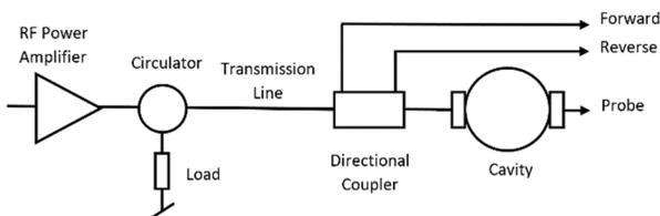
Figure 1: Traditional SRF cavity RF circuit.
