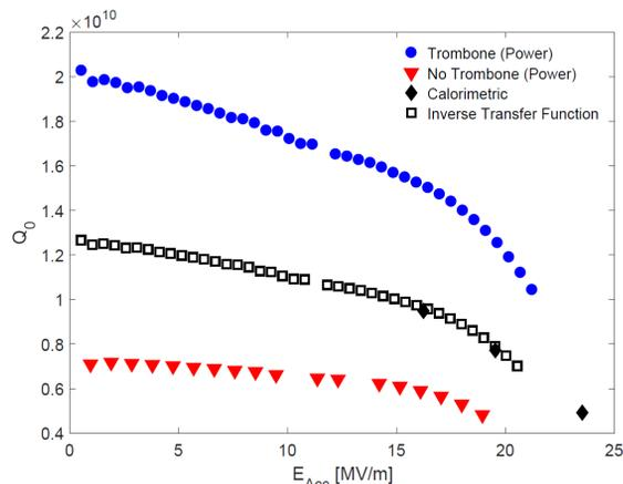
Figure 6:  $Q_0$  vs  $E$  measured by power with no trombone (Red Triangles), at the zero trombone position (gives 'maximum  $Q_0$ ') (Blue Circles), and as measured with Transfer Functions (Black Squares) compared with calorimetric measurements (Black Diamonds).
