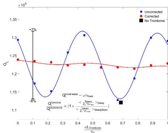
Figure 2: Loaded Quality Factor  $Q_L$  vs trombone length (Blue Squares).  $Q_L$  measured without the trombone circuit (Black Diamond). Using directivity-corrected powers, the measured  $Q_L$  can be corrected (Red Circles).
