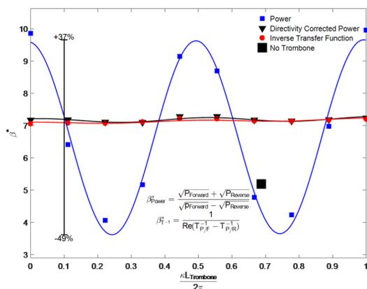
Figure 5: Measured  $\beta^*$  via power measurements versus trombone angle with uncorrected signals (Blue Squares) and directivity-corrected signals (Black Triangles) compared to directivity-corrected Transfer Functions (Red Circles)..
