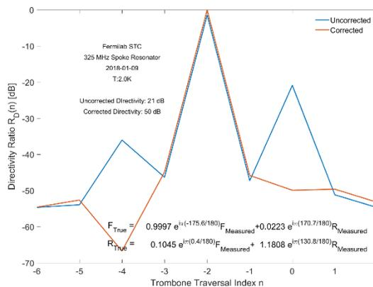
Figure 3: Directivity determination before and after correction factor applied.
