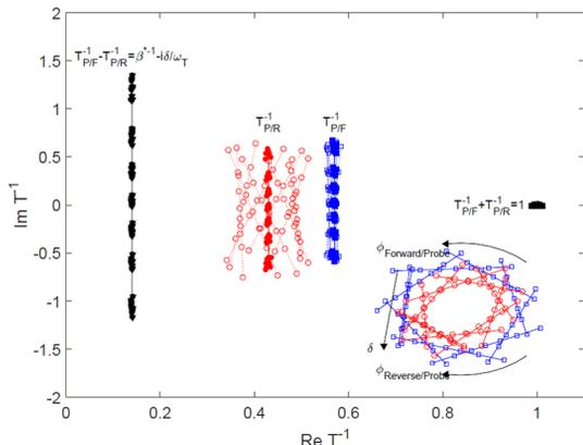
Figure 4: Inverse Transfer Functions (F/P & R/P) including sums and differences. Blue squares are F/P, red circles are R/P, and black triangles are the sums/differences. Closed symbols use directivity-corrected signals, and open symbols are uncorrected. Inset data (lower right) shows data before calibration/directivity correction.
