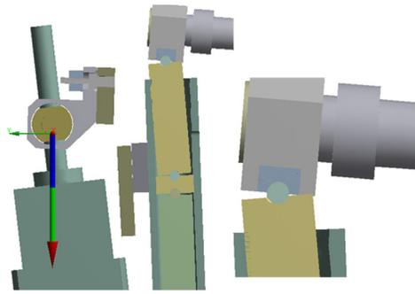
Figure 4: Displacement of the piezo tuner components with forces applied to the tuner.
