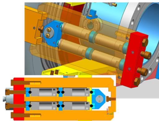
Figure 2: 3-D model of the fast tuner built from 4 piezo-actuators installed inside cartridge.
