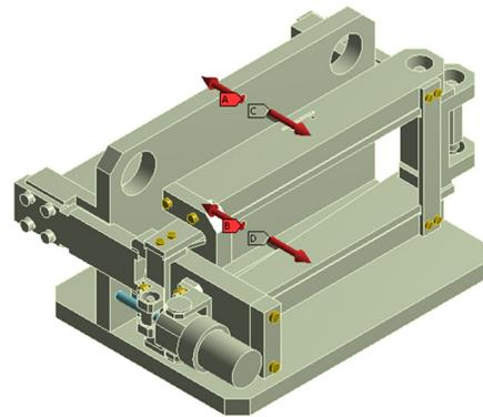
Figure 5: ANSYS model of the tuner, mounted on the test stand. Gravity forces considered during calculations of the stiffness Top & Bottom tuner arms.
