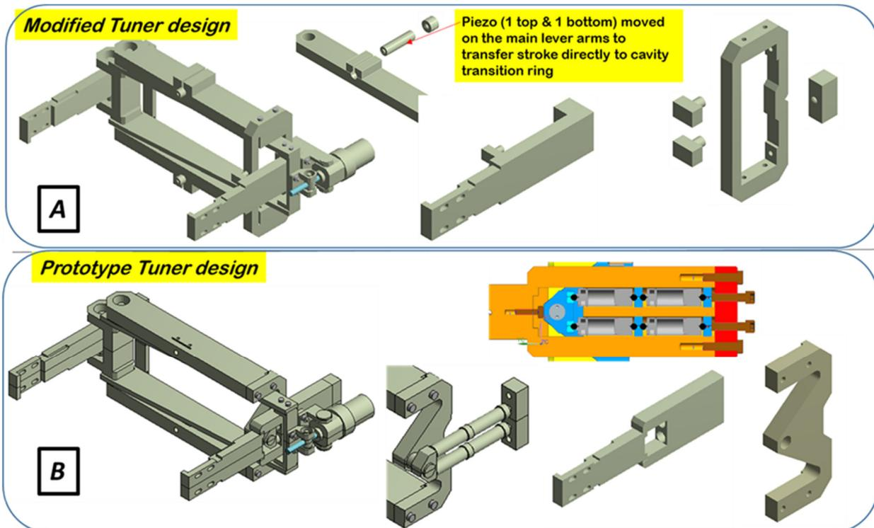
Figure 6: New vs Modified Tuner Design.
