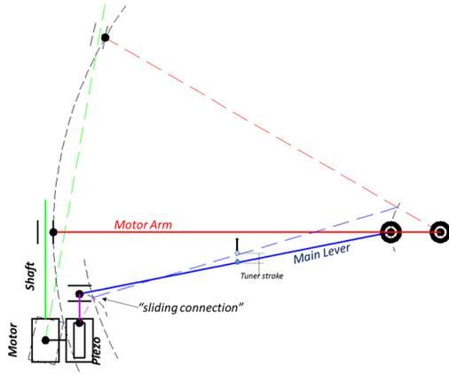
Figure 3: Kinematics scheme of the double lever tuner. Left end of the main lever required “sliding connection” for operation of the double lever scheme.
