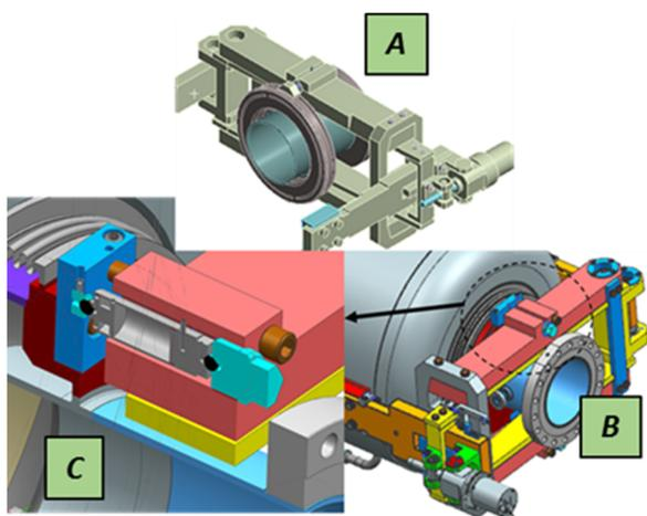
Figure 7: 3-D model of the modified tuner (A&B). (C) - Piezo-actuator inserted into main tuner arm and interfaced cavity through Nb-Ti ring.
