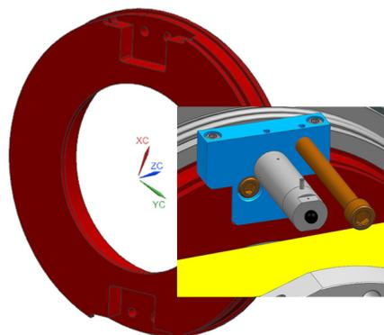
Figure 8: Nb-Ti interface ring that welded to cavity beam-pipe. Insert: Piezo-capsule, safety rod and interface plate that attached to Nb-Ti ring.
