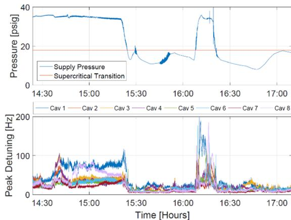
Figure 2: Supply helium criticality transition. Top plot is helium supply pressure, bottom plot is cavity peak detuning.
