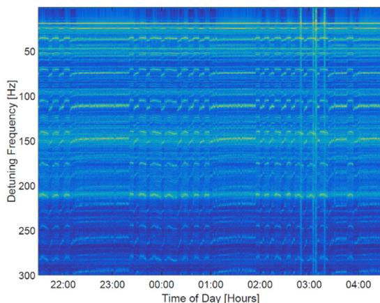
Figure 1: Spectrogram of the captured detuning of cavity 1 on the FNAL pCM (F1.3-01), 2017/01/10. 7 hours of continuous capture at 2 MV/m in SEL mode. Cryogenics in default configuration.
