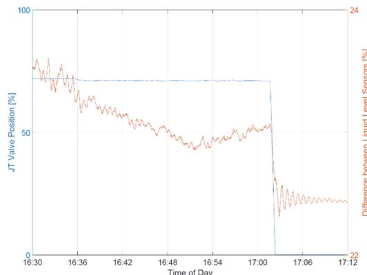
Figure 5: Change and oscillation in differential liquid level after helium flow was stopped.
