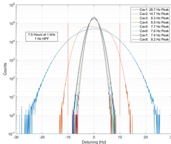
Figure 4: F1.3-02 detuning histogram. 7.5 hours of continuous data measured at low field in SEL. Includes TAO improvements including flow direction and stem wipers on all valves. LCLS-II specification is plotted as vertical red lines.
