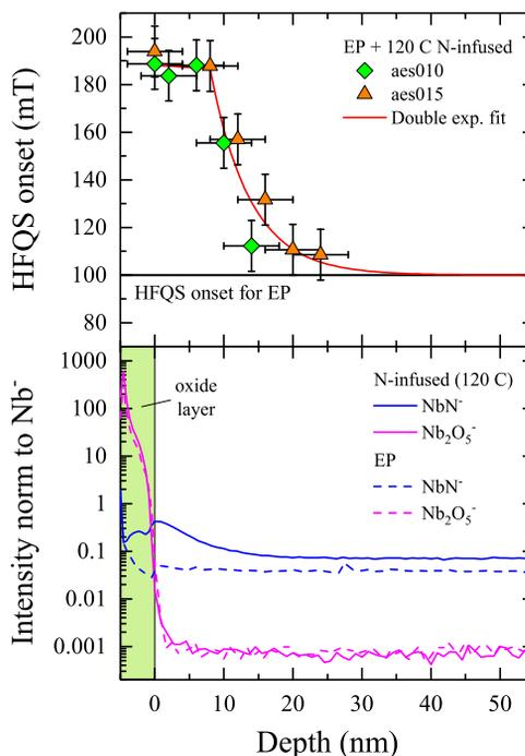
Figure 3: The HFQS onset data as a function of material removed compared to the nitrogen concentration profile measured with TOF-SIMS on cavity cut-outs. The RF data reported from zero up to ~10 nm correspond to the maximum field reached by the cavity (quench field) since HFQS was not observed.
