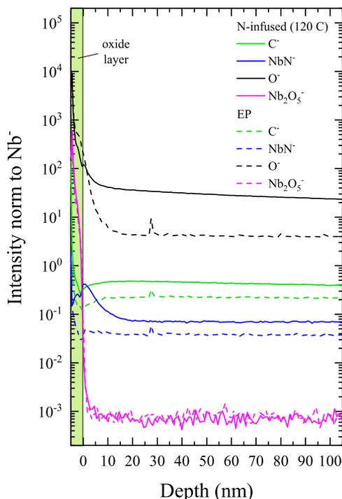
Figure 2: Comparison between TOF-SIMS data for the 120 °C N-infused and EP cavity cut-outs.
