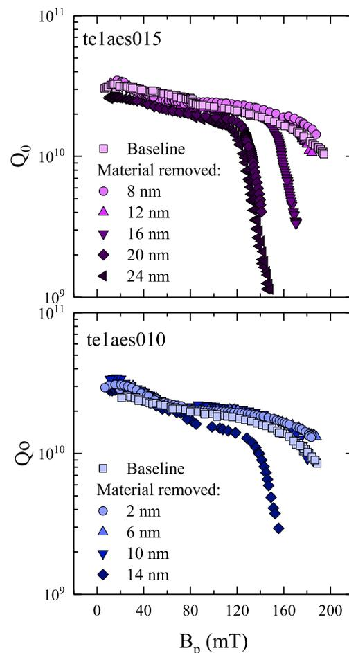
Figure 1: Q-factor versus peak magnetic field of the two cavities studied (te1aes010 and te1aes015) after successive material removals via HF rinsing.
